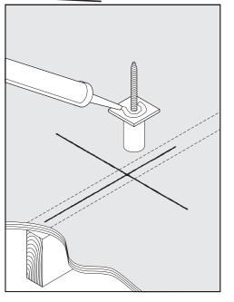
**STEP 2:** Apply a generous amount of Polyurethane sealant (Sikaflex<sup>TM</sup> 1A or equivalent) to the bottom of the seal plate of the Foam-Jack<sup>TM</sup> creating a circle around the lag bolt hole.
