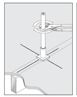
**STEP 4:** Install post using an adjustable wrench turning clockwise until fully secured. Avoid twisting the base while tightening.
