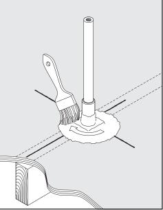
**STEP 5:** Seal the top of the seal plate with a layer of Sikaflex<sup>TM</sup> using a stiff paintbrush. Be sure to cover the entire base plate, at least half the post and about 1- $1/2^n$  around the plate.
