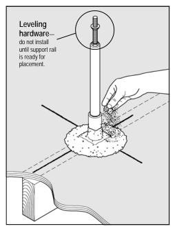
**STEP 6:** Using Play/Silica sand, cover the sealant. This step prevents debris from sticking to the sealant while drying and gives it a clean, finished appearance.
