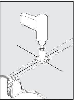
**STEP 3:** Using a cordless impact and a 9/16" deep socket, install the bolt into the Foam Jack<sup>TM</sup> base. Be sure to allow the sealant to flow outward around the edges of the seal plate.
