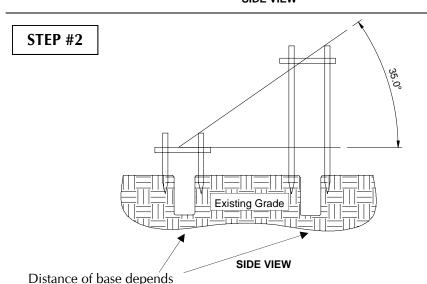
Determine the proper angle for the module array and install grade stakes as illustrated (left), do not exceed 5 ft. of vertical post length from grade.
