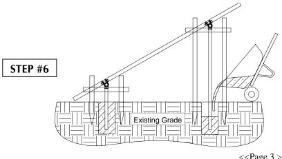
Align the end of the channel using a string line. Tighten all the "U-Bolt" assemblies and re-check alignment the vertical pipe supports. You are now ready to pour concrete into the footings. Tap the concrete to ensure contact with the vertical pipe support. Remove the support bracing after the concrete has set. You are now ready to install your modules.
