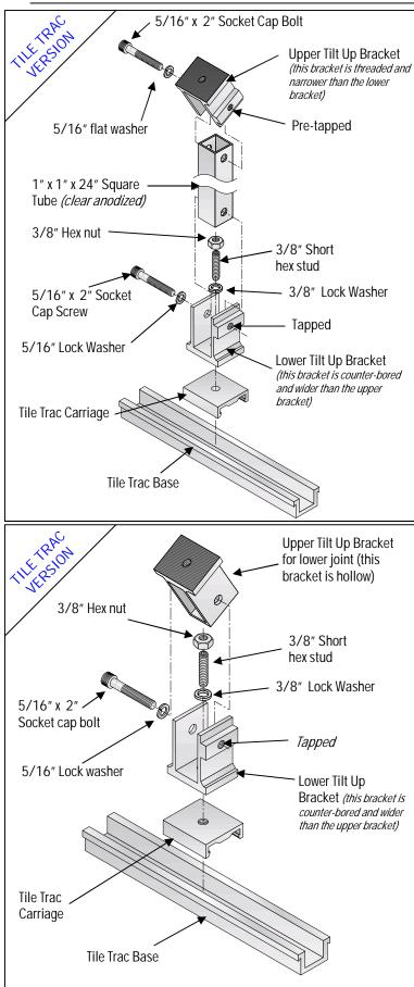
STEP 1–USING TILE TRAC ATTACH THE REAR ASSEMBLY:
