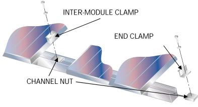
Please note that all module end clamps are proprietary and specially extruded to fit a specific brand of module. Since many of these tolerances are very small, we install a die line (marker) to differentiate the correct die per module frame.
