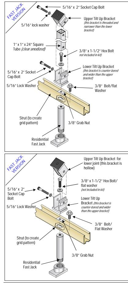
STEP 1-USING FAST JACK ATTACH THE REAR ASSEMBLY:
