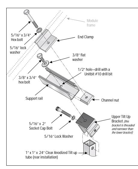
STEP 3–ATTACH THE SUPPORT RAILS (not included in tiltup kit) TO THE TILT UP ASSMBLY:
